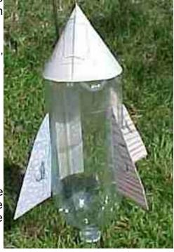
Fins should be constructed of a firm material (e.g. rigid cardboard) and be well-secured to the bottle (e.g. with duct tape). The size of the fin does matter! Think what kind of fin works best on paper airplanes. Cut the fins first but add them last so that they don't bend during construction.
